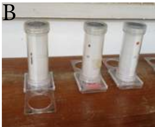
B – World Health Organisation insecticide susceptibility kit used for measuring insecticide resistance status of mosquitoes
