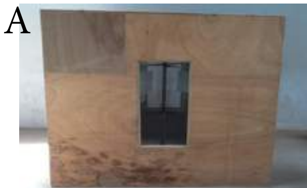
A – Peedy grady chamber used to evaluate efficacy of mosquito coil against mosquitoes
